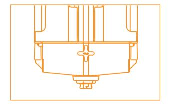
(3) Loop the waterfall mounts on the wire deck or cross bar. Slightly separate the mounting hardware until the hooks slide into the holes on the side of the power supply enclosure.
