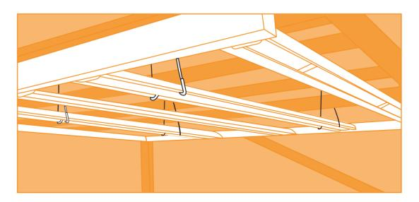
Note: Do not attach mounting hardware to the end light bars, else you may risk damaging the fixture.
